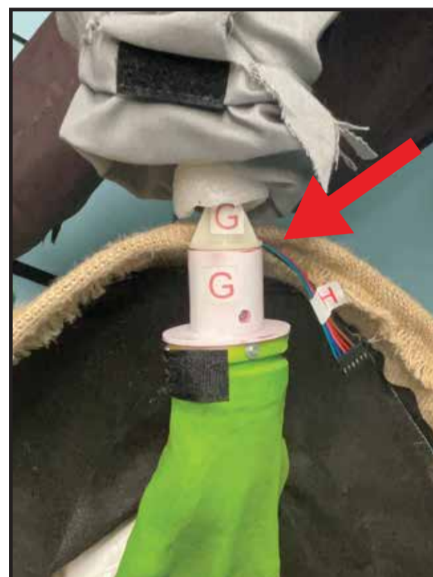
14. Snap lock the right arm on the BODY AND HEAD to the SKULL AND HAND. Match G to G
