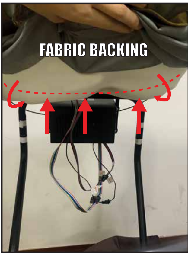
9. Secure the hook and loop strip located under the fabric backing around the FRONT edge of the WAIST BRACKET.
