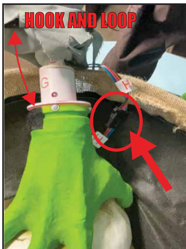
15. Connect the wire from the CONTROL BOX to the wire on the SKULL AND HAND. Push wire up the sleeve and secure hook and loop fastener. Match H to H
