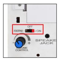
Move the switch to the ON position. Make a loud sound (clap) or move in front of the item to activate.
