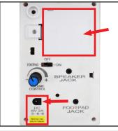
10. Insert 4 AA batteries (not included) into the battery compartment. OR Insert the 6V 2A DC ADAPTER into the CONTROL BOX (included).
